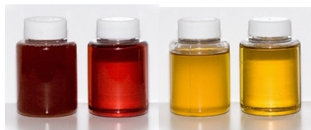
Diesel Fuel Hydraulic Oil Before and after filtration
