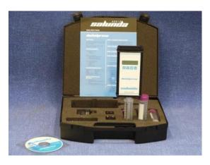
The FAME tester displays results in % from 0-100% of the biofuel
